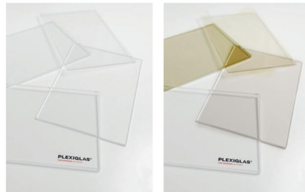
Fig. 1: PLEXIGLAS® compared to other plastics in unused condition.
